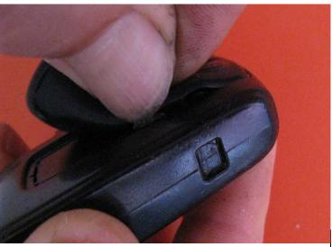
Once first button sits in properly in the cut out, you will repeat the same fitting process for the second and third cut out.
