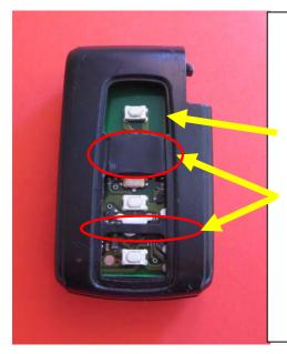
With flat screwdriver lift sides of the soft rubber pad and remove it from the shell. Do not insert screwdriver inside the shell as you may damage electronic switches.
