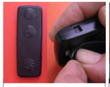
Start fitting pad from the **top** (**lock button cut out**) by slightly bending and sliding it under the sides of the cut out.
